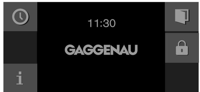
The child lock is activated. The standby screen appears. The
