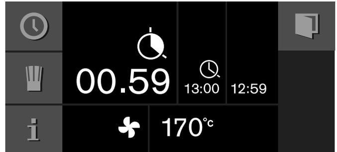
The appliance switches off after the cooking time has elapsed. The ⌚ symbol flashes and a signal sounds. The signal stops when you touch the ✓ symbol, open the appliance door, or switch the function selector to 0.
