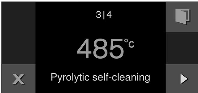
A signal sounds after 3 hours. A message appears in the display. Once the appliance has cooled down, wipe the remaining ash out of the interior with a moist cloth.
